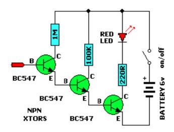
This circuit is so sensitive it will detect "mains hum." Simply move it across any wall and it will detect where the mains cable is located. It has a gain of about  $200 \times 200 \times 200 = 6,000,000$  and will also detect static electricity and the presence of your hand without any direct contact. You will be amazed what it detects! There is static electricity EVERYWHERE! The input of this circuit is classified as very high impedance.
