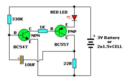
This is basically a high gain amplifier with feedback that causes the LED to flash at a rate determined by the 10u and 330k resistor. Remove one of the transistors and insert the unknown transistor. When it is NPN with the pins as shown in the photo, the LED will flash. To turn the unit off, remove one of the transistors.
