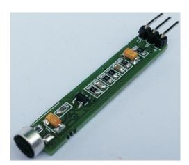
The single supply microphone pre-amplifier amplifies the output signal of an electret capsule microphone to audio line levels. An op amp is used as a trans-impedance amplifier to convert the output current from the microphone in to a signal level voltage. The circuit works with 9V so it is good choice for battery operated systems.
