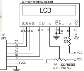
This Project PCB will help you connect a standard 16x2 backlight Alphanumeric LCD to any of your microcontroller project in the 4 bit mode.
