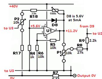
U1 circuit is a simple voltage reference. It uses an opamp U1 to amplify a 5.6V zener diode by a factor of 2, due to the ratio of R5 and R6, to 11.2V
