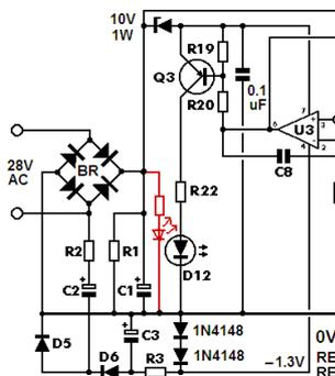
**Q:** Hi, I am facing the problem Please help me out. At the output of U1 I get 11.8V and at the output of U2 I get 34V. But at pin 2 and pin 3 of U3 is 14.2V and 15V respectively. R3 gets heated up and I replaced three times already. Across the load resistor (20W, 10K) I get 41V and the same voltage is across the output of bridge and output voltage is not varying by 20K pot.
