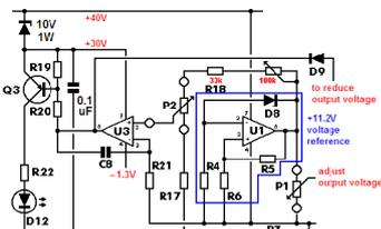
U3 controls the current regulation. P2 sets the current and P1 sets the voltage.
