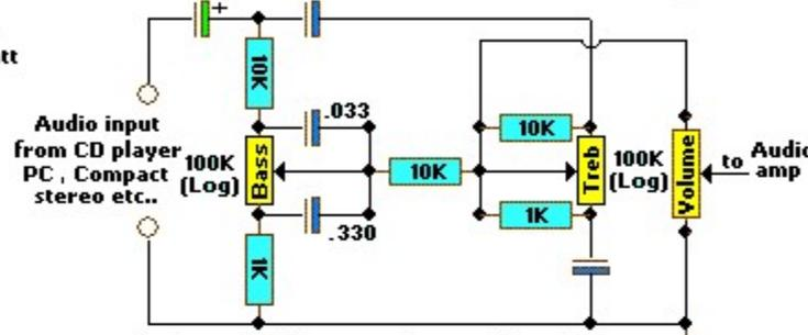
This circuit diagram is for one channel. If two channels required so build it two times.
