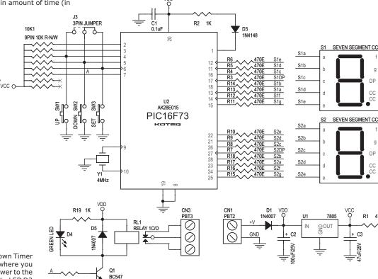
CN1 Connector: Power Supply Input 12 VDC D2 LED: Power-On Indication
