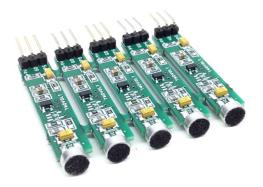
The single supply microphone pre-amplifier amplifies the output signal of an electret capsule microphone to audio line levels. An op amp is used as a trans-impedance amplifier to convert the output current from the microphone in to a signal level voltage. The circuit works with 9V so it is good choice for battery operated systems.
