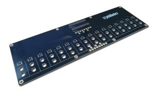
The Array-SL board enables releasable connections of LED strips with the Pixblasters MS1 Video LED Controller and an easy build of the LED matrix. It distributes the video control signals from the MS1 LED controller and the power sourced from an external power supply. The board includes holes for easy wall mounting.
