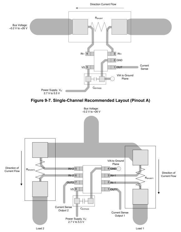
Figure 9-8. Dual-Channel Recommended Layout (VSSOP)
