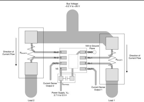
Figure 9-9. Dual-Channel Recommended Layout (WSON)
