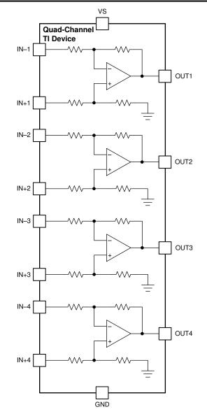
Figure 8-3. INA4180 Functional Block Diagram
