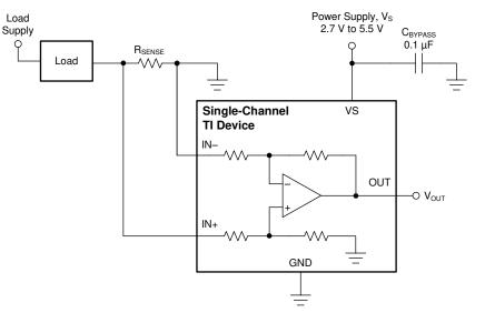
Figure 9-3. Low-Side Sensing
