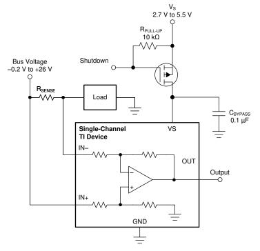
Figure 8-6. Basic Circuit to Shut Down the INxA180
