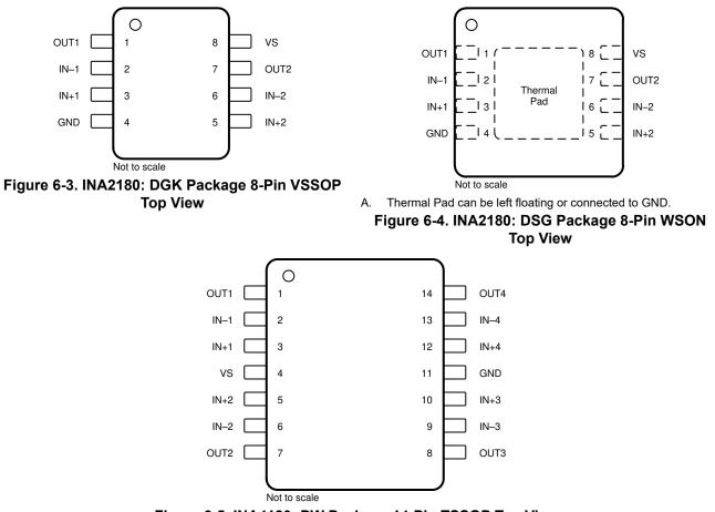
Figure 6-5. INA4180: PW Package 14-Pin TSSOP Top View
