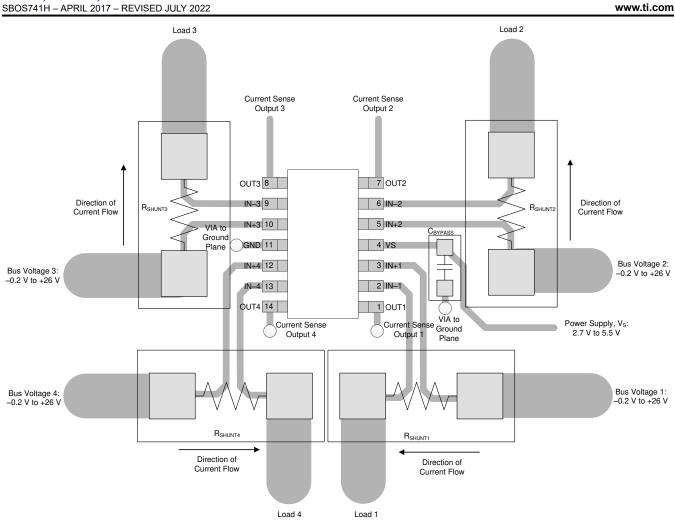
Figure 9-10. Quad-Channel Recommended Layout
