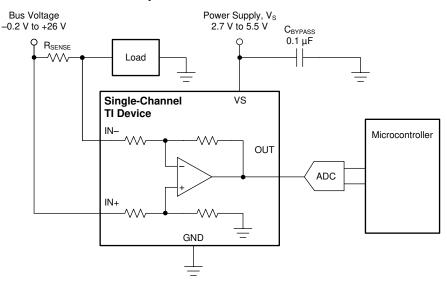
NOTE: For best measurement accuracy, connect analog-to-digital converter (ADC) reference or microcontroller ground as closely as possible to the INAx180 GND pin, and add an RC filter between the output of the INAx180 and the ADC. See *Closed-Loop Analysis of Load-Induced Amplifier Stability Issues Using Z<sub>OUT</sub>* for more details.
