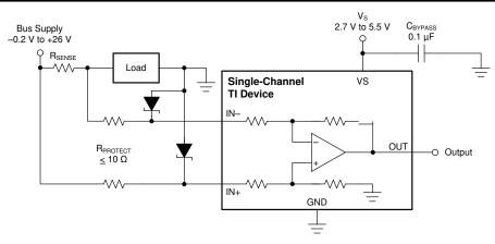
Figure 9-5. Transient Protection Using Dual Zener Diodes
