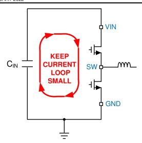
Figure 11-1. Current Loops with Fast Edges
