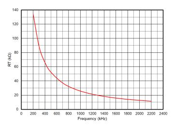
Figure 8-3. R<sub>T</sub> Versus Frequency Curve
