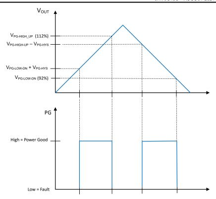
Figure 8-5. Static Power-Good Operation
