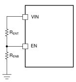
Figure 8-2. System UVLO by Enable Divider
