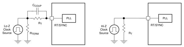
Figure 8-4. Synchronizing to an External Clock
