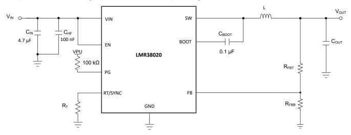
Figure 9-1. Example Application Circuit
