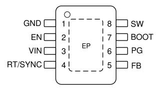
Figure 6-1. 8-Pin SO PowerPAD DDA Package (Top View)
