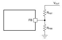
Figure 8-1. Output Voltage Setting
