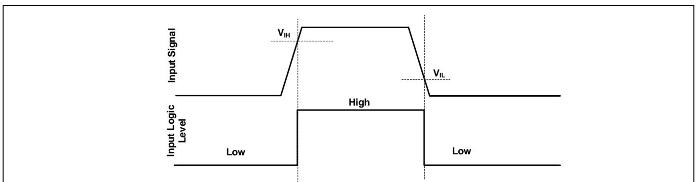
**Figure 12** HIN & LIN input thresholds
