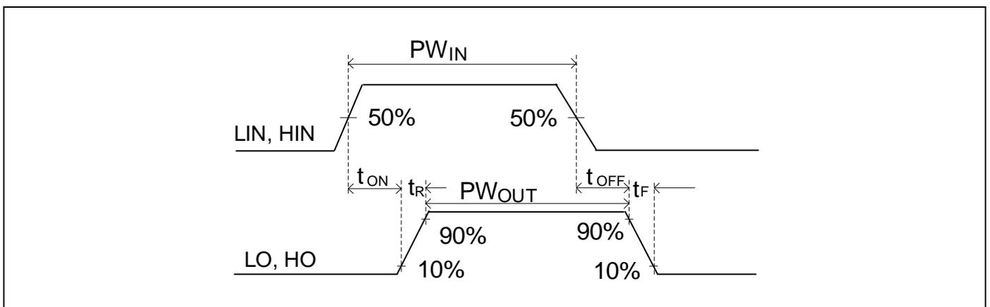
Figure 6 Switching timing waveforms \_ Input/output timing diagram
